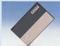
IC Card JEIDA (Ver 4. 1) memory card to record graphics and other printing information
